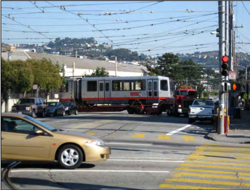
Figure 40: Truck Carrying a Two-car LRV on its Truck Bed Exiting the Driveway South of the Proposed San Jose Platform
