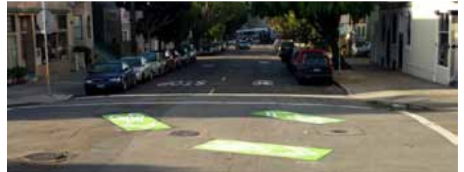
Sharrows/Painted Sharrows: On-street markings placed in the travel lane to indicate to motorists and riders that the lane is shared with people on bicycles, and that both may use the full lane.
