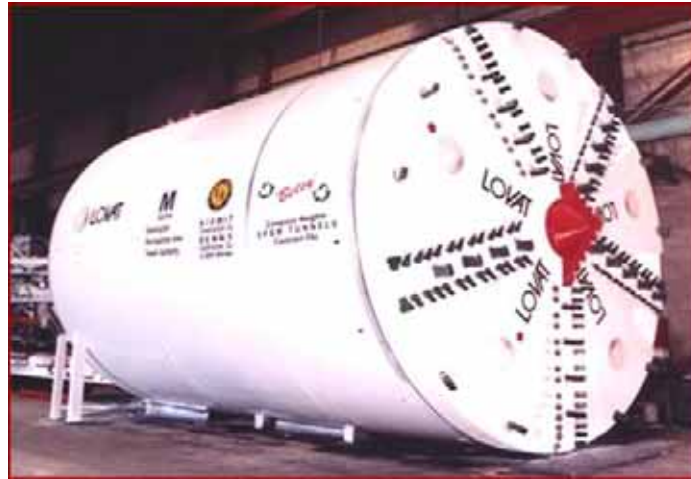
Figure 3-5: Tunnel Boring Machine
