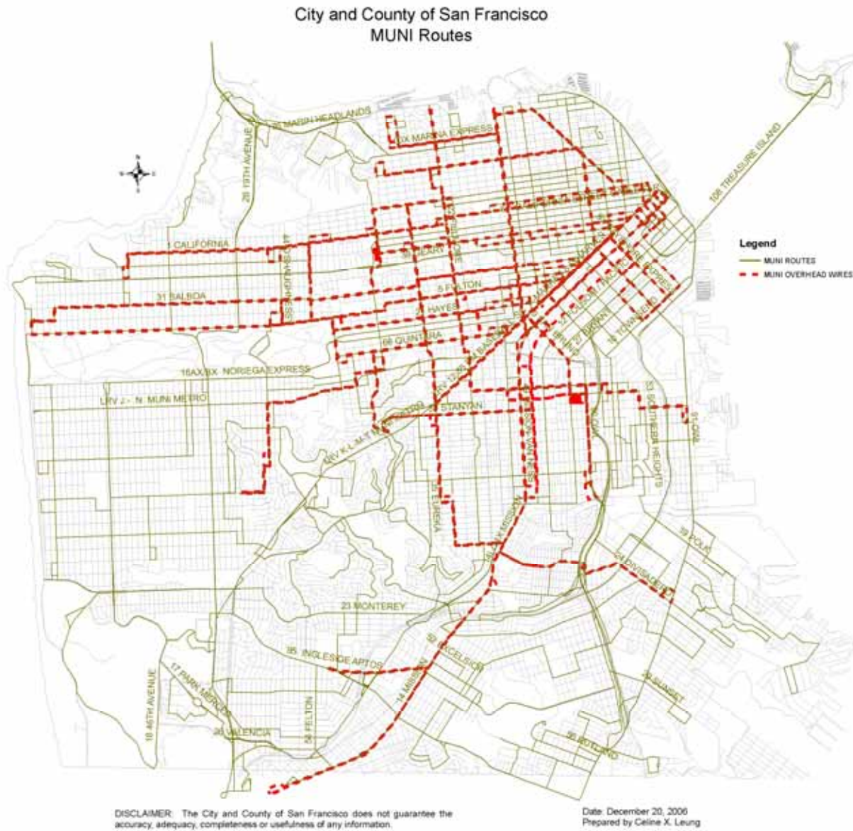
Figure 8-3: Existing Trolley Overhead Lines
