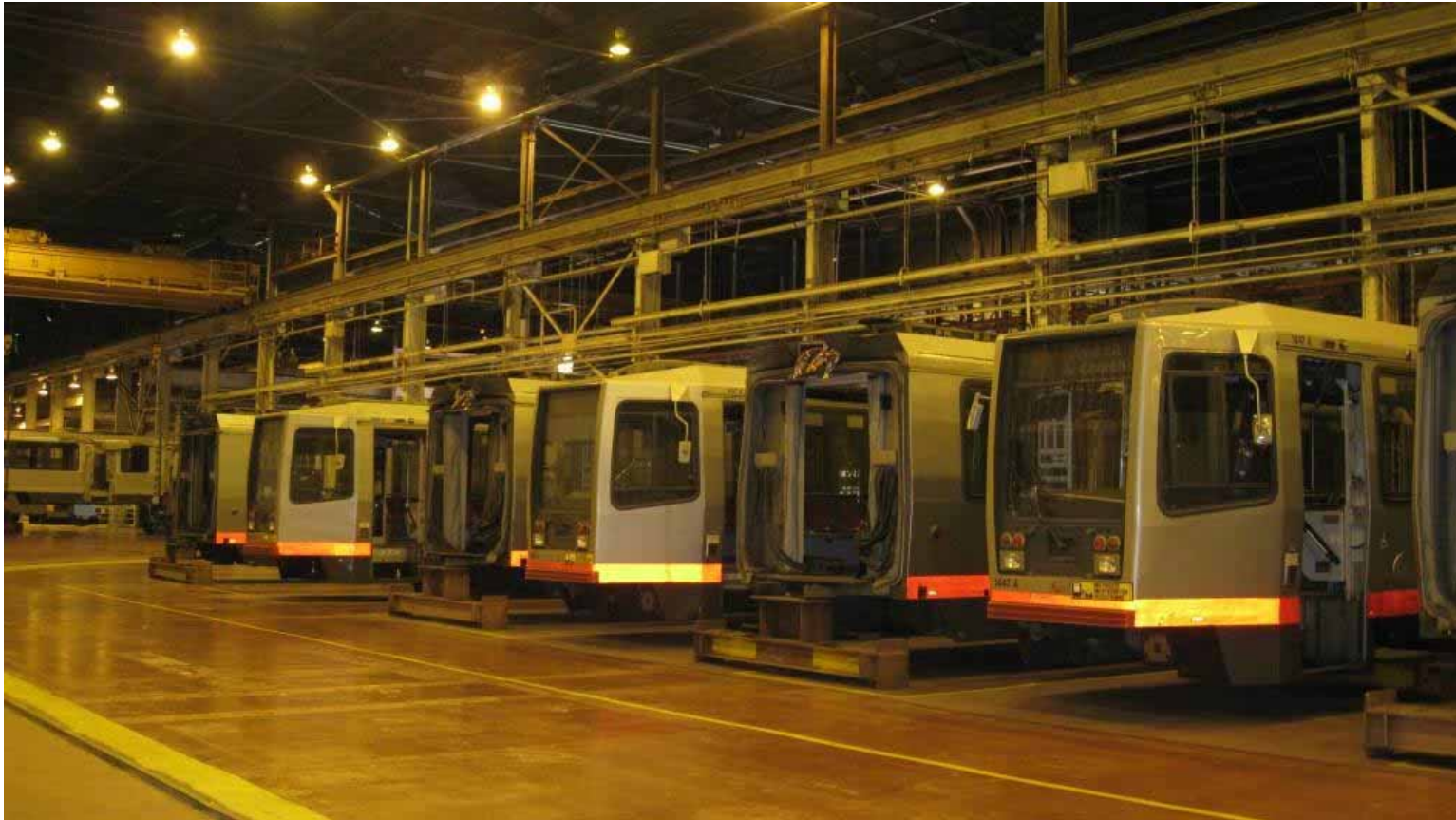
CARS DISASSEMBLED AND COMPONENTS SENT OUT FOR REBUILD
