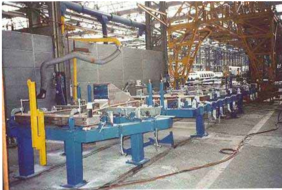
Figure No. 1 – SFMTA Breda Car underbody structure being assembled using the assembly fixture
