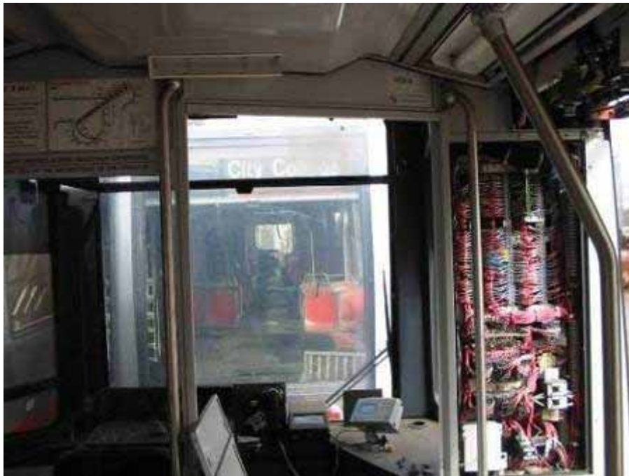
Figure 4 – Picture of missing panels and wiring harness from LRV 1429
