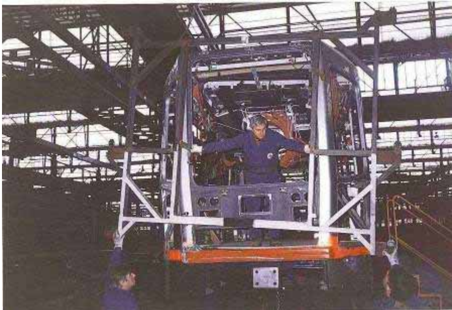
Figure No. 2 – LRV No. 1407 being aligned using an alignment fixture
