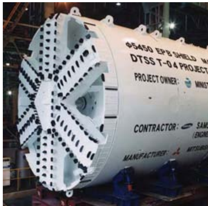
Figure 8: Tunnel Boring Machine
